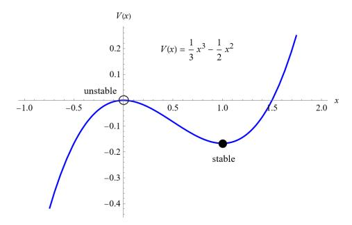
The graph of V(x) versus x is to be thought of as a two-dimensional rollercoaster. A particle on the curve at  $x^* = 0$  is unstable because the slightest nudge in either direction will send it away from  $x^* = 0$  indefinitely. A particle on the curve at  $x^* = 1$  that's nudged in either direction will return to  $x^* = 1$  because it's stable.
